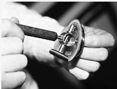
**Joe's newly-made thorn polishing tool is based on an original design**
